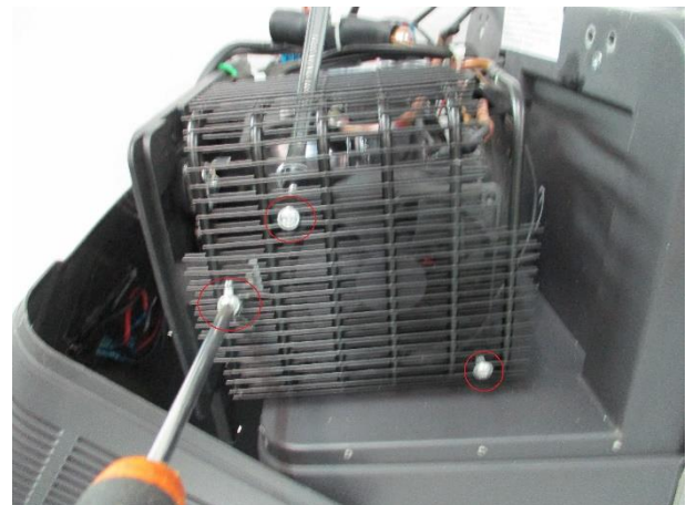
4. Unscrew the bolts from each side (6 bolts)
