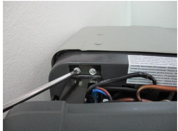
2. Unscrew the two brackets
