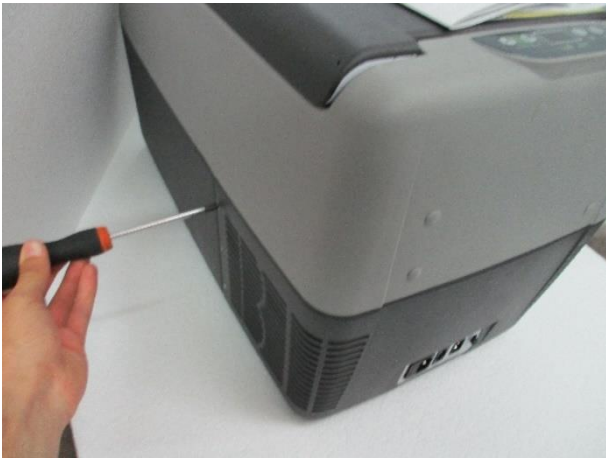
1. Unscrew the plastic support (11 screws)
