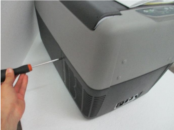
1. Unscrew the plastic support (11 screws)
