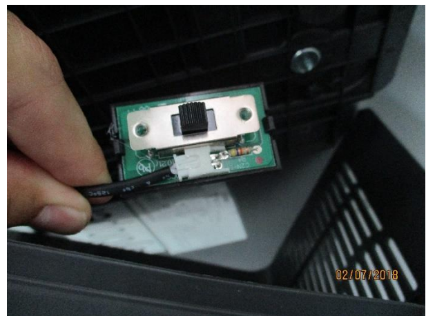
4. Remove the switch and reverse the procedure to install a new one
