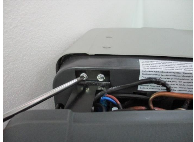
2. Unscrew the two brackets
